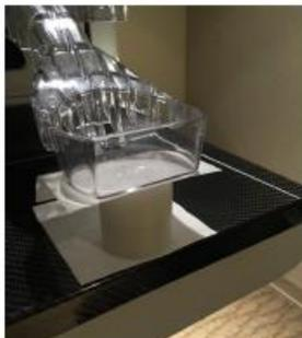
Figure 6. Position and compression of compression thickness indicator phantom using spot compression paddle.
