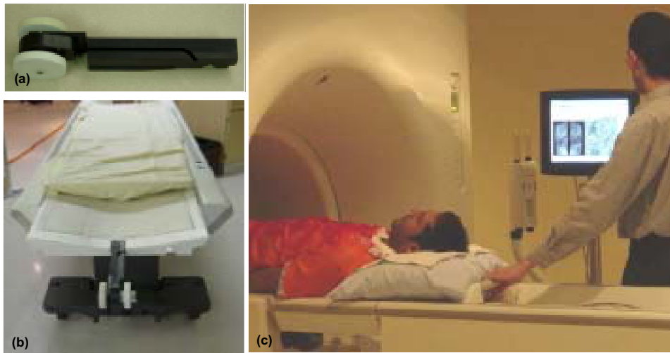
Figure 4: (a) Custom-designed position encoder module and (b) how it is mounted to the end of patient table. The position-encoding system provides position information to the workstation in real-time. (c) The operator interacts with the scanner via a “floating” table according to the visualized contrast dynamics displayed on an in-room, MR-compatible monitor [24].
